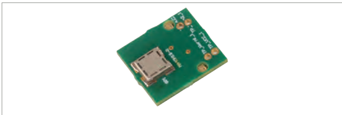
Abb. 2: The Ultrasonic circuit board transmits signals above the audible frequency range that are used by the system to determine the vehicle's position.
