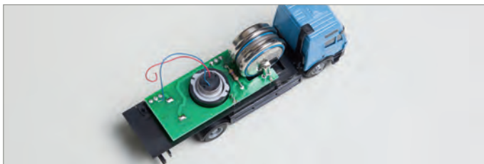
Abb. 29: Truck model with universal circuit board, plug-in batteries, no wiring
