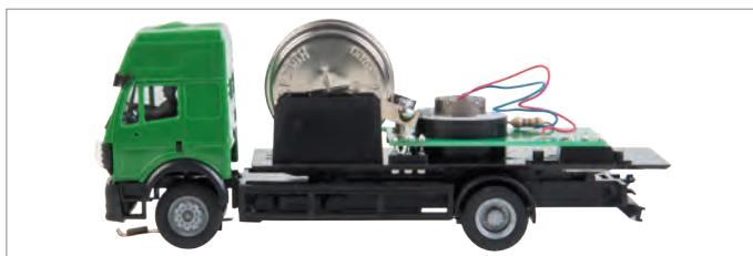
Abb. 21: Truck model, soldered batteries, side view
