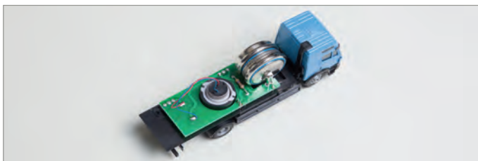
Abb. 9: Car System truck model with universal circuit board, plug-in batteries
