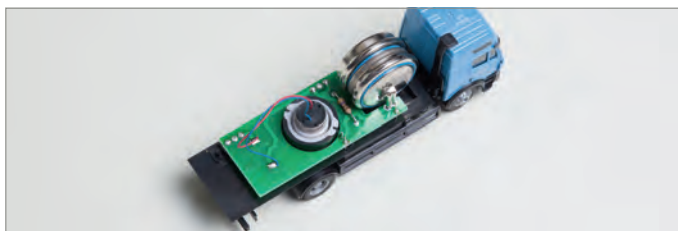
Abb. 28: Truck model with universal circuit board, plug-in batteries, and wiring
