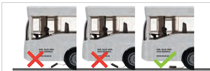
Abb. 51: Adjusting the guide wheel
