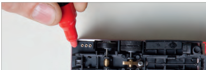
Abb. 10: Mark the polarity of the charging port on the outside of the vehicle housing
