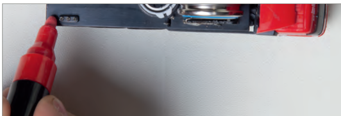
Abb. 11: Mark the polarity of the charging port, inside the vehicle housing
