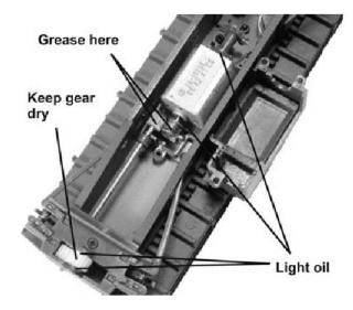
Apply a small drop of light oil for electric motors to the bearings; apply a light gear lubricant to the gear train as shown.
