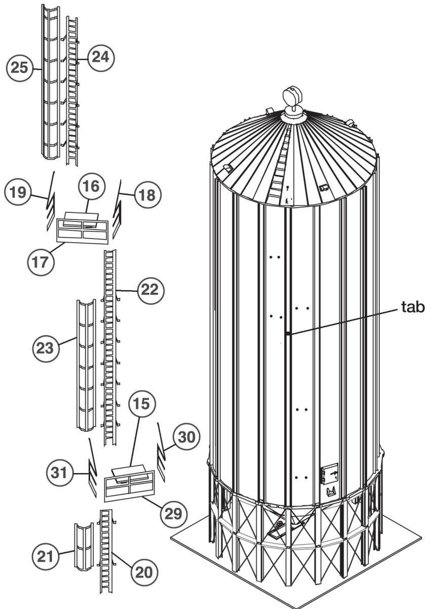
8. Glue the ladders (20, 22, 24) to the cages (21, 23, 25) respectively and then into the holes in side #10.
