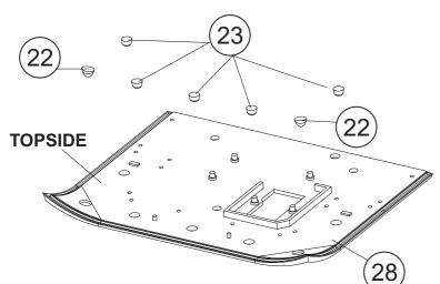
2) Press Lamp Fixtures (22, 23) into the locations shown in Ceiling Assembly (28). The Fixtures should be flush with the top surface of Part 28. Note: Part 22 has a curve cast into the top that matches the corner curve. When installed properly, the curves align to form a smooth surface. Secure each Fixture with a small drop of glue.
