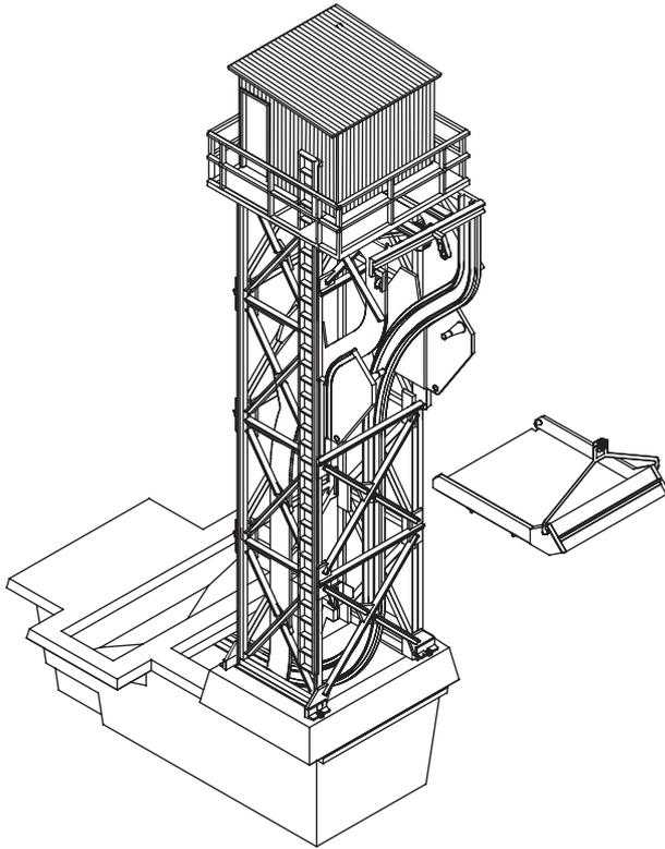
13. Snap completed chute into the holes on the inside of the sides. Note: If you wish to rig the chute follow the chute rigging instructions.
