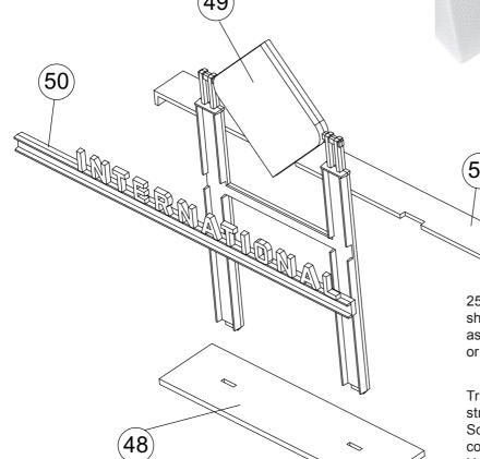
25. Assemble the International sign as shown (48, 49, 50 & 51). Center the Sign assembly in front of the Entrance on Wall 9, or where desired.
