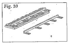
Chamfer the exposed corner in order to clear the wing nut. Repeat the process for the other support.
