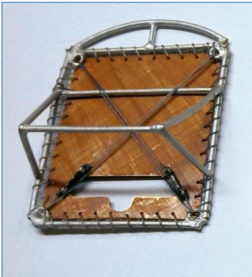
Figure 2.4 Frame 5 with Cockpit Rear Wall
