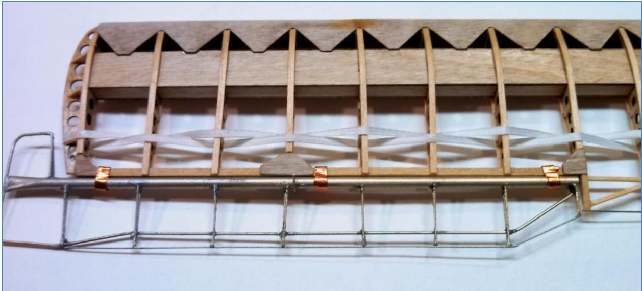
Figure 1.17 Aileron Mounted to Wing
