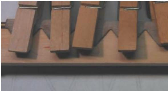
Figure 1.8 Leading Edge Clamped on Jig
