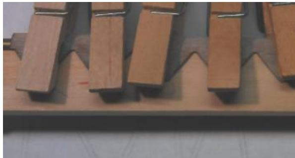
Figure 1.8 Leading Edge Clamped on Jig
