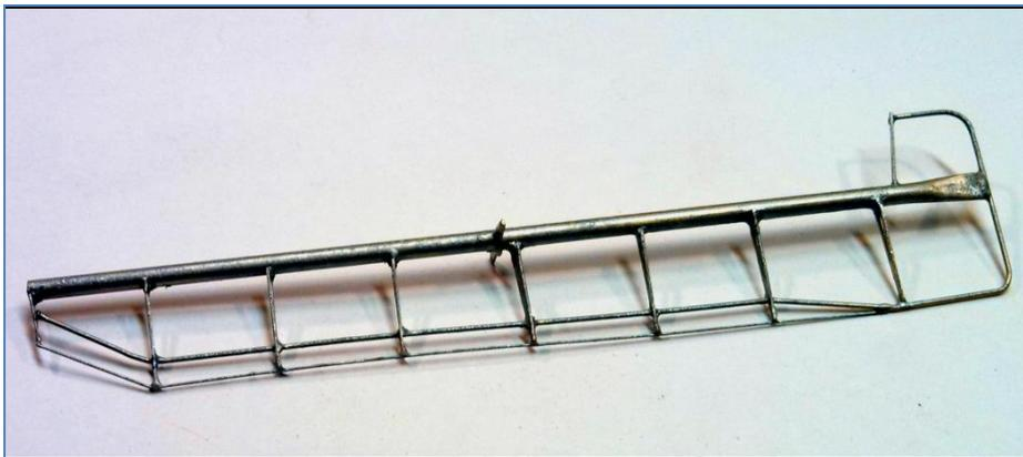
Figure 1.16 Completed Aileron
