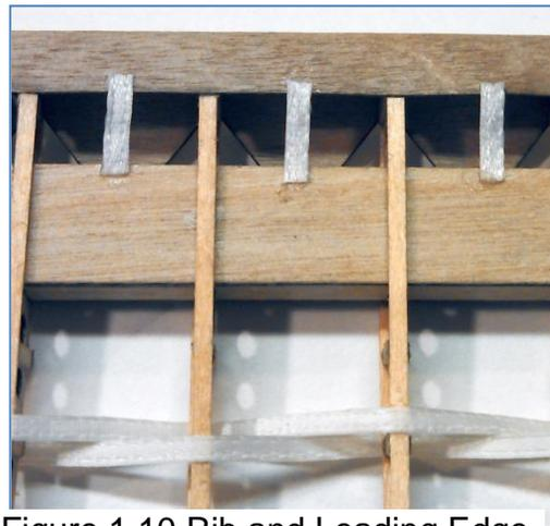
Figure 1.10 Rib and Leading Edge Bracing
