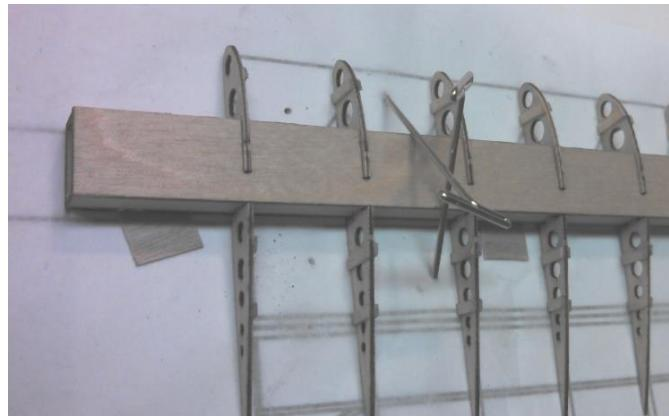
Figure 1.5 Building the Wing Detail
