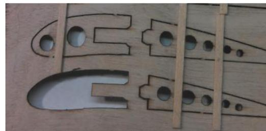
Figure 1.4 Rib Stiffener Details
