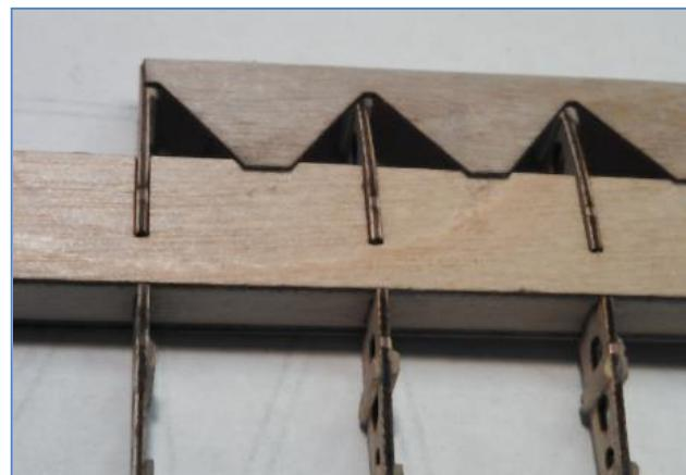
Figure 1.9 Leading Edge Gluing Detail
