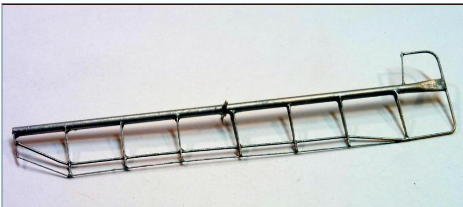
Figure 1.16 Completed Aileron
