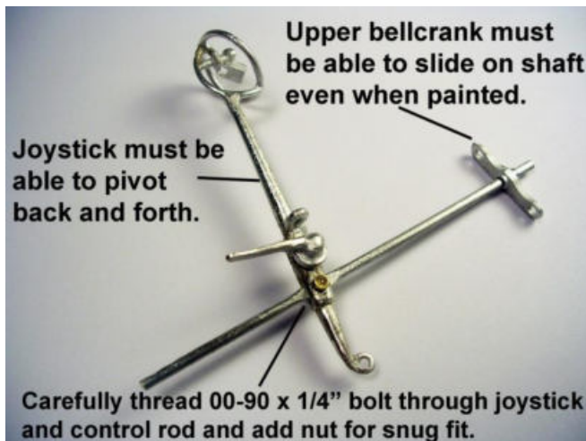
Index shaft into rear hole location and then index into front hole location, then with joystick vertical glue bellcrank on shaft parallel to ground against baffle.
