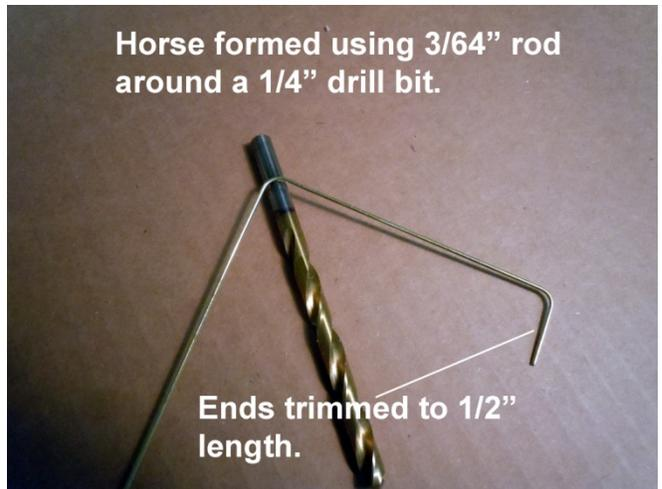
Horse formed using 3/64" rod around a 1/4" drill bit.
