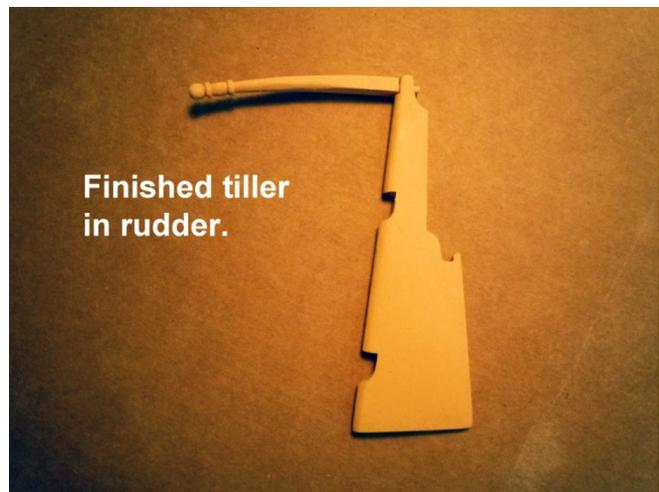
Finished tiller in rudder.
