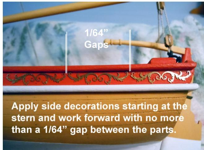
Apply side decorations starting at the stern and work forward with no more than a 1/64" gap between the parts.
