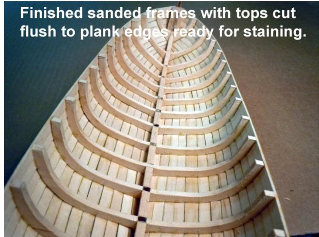
Once sanding is completed now apply wood conditioner to the entire inner hull surfaces including **Keel**, bow and **Transom** (see Plan Sheet) surfaces. When dry then apply two (2) coats of Natural Stain with no need to wipe with cloth. After the first coat is applied if any imperfections need to be sanded or cut away like fussy edges from sanding do so before applying the second coat.
