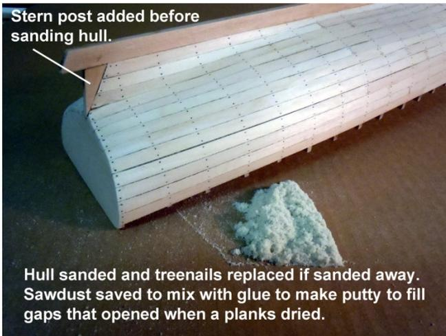
Once smooth then use 120 grit sandpaper for a light finish sanding. To work around the curve make short sanding sticks using 1/4" and 1/2" wood dowels with sandpaper glue to them. These will be handy working around the stern post and blending the **Garboard** (Plank #1) to the keel and stern post. When finished again check the treenail marks and add as necessary. All the treenails should look the same prior to adding the Wood Conditioner.
