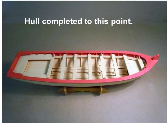
The bow **Breast Hook (1)** will need to have the front curved mating surface sanded to fit the **Cap Rails**. Sand the curved forward edge at a slight downward angle for a tighter fit.
