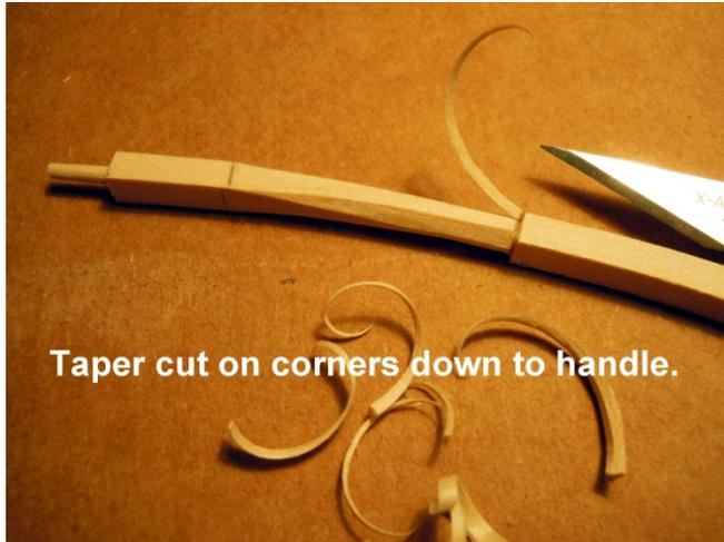
Taper cut on corners down to handle.
