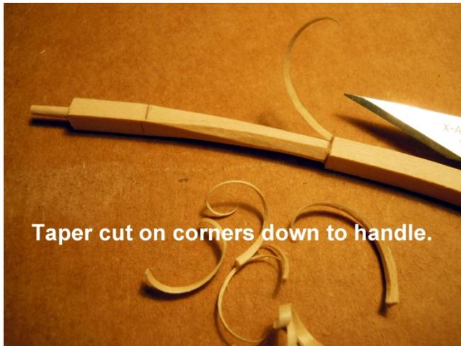
Taper cut on corners down to handle.
