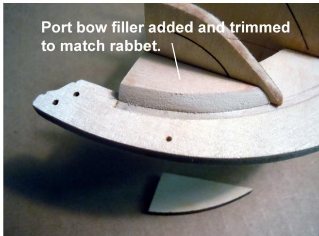
Remove the laser cut **Bow Fillers** from the carrier sheet and sand the two straight edges to remove the laser char. Then very carefully carve an angle on the curved edge to match the laser cut line along the rabbet edge. There will be a left and right so make sure to carve the correct curved edges. Do one at a
