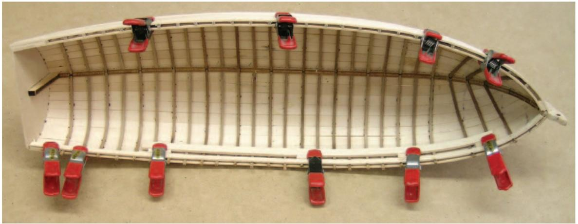
*Photo 20, forming the thwart risers to shape*
