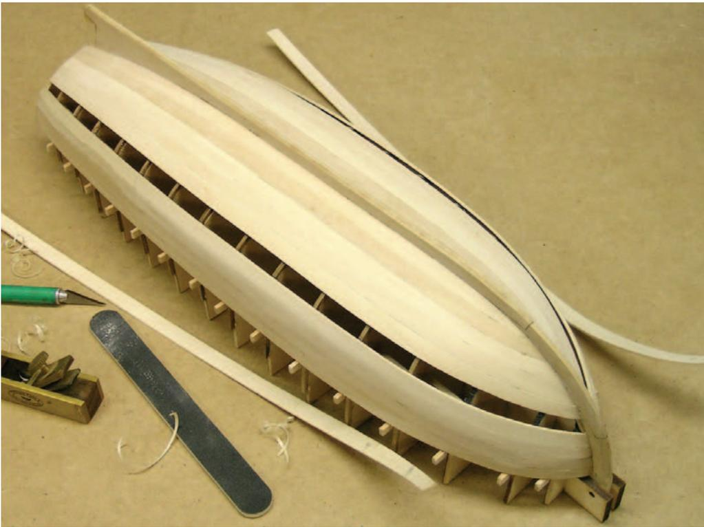
Begin fitting the shutter planks at the bow. Sand both edges of the plank until it fits at the bow. Continue along the length fitting a little at a time until the whole plank will drop in. The planking is done, time to sit back and admire your work.
