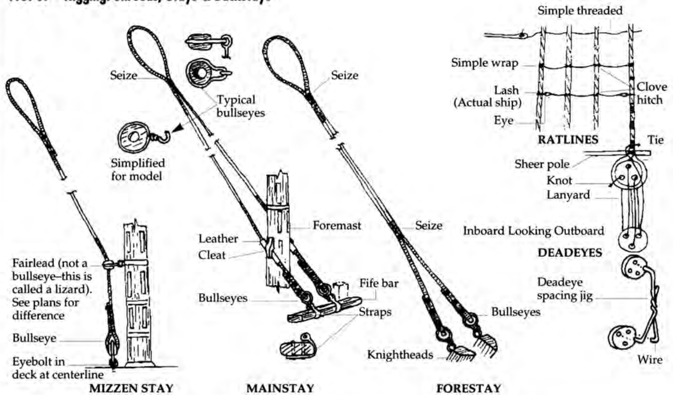
FIG. 87 - Rigging: Shrouds, Stays & Backstays
