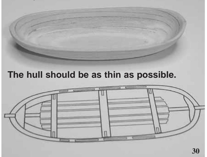
The hull should be as thin as possible.
