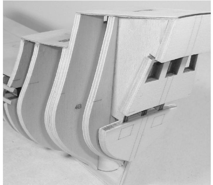
*False decks are in position and the hull is faired. The bulkhead edges are beveled more severely at the bow and stern*
