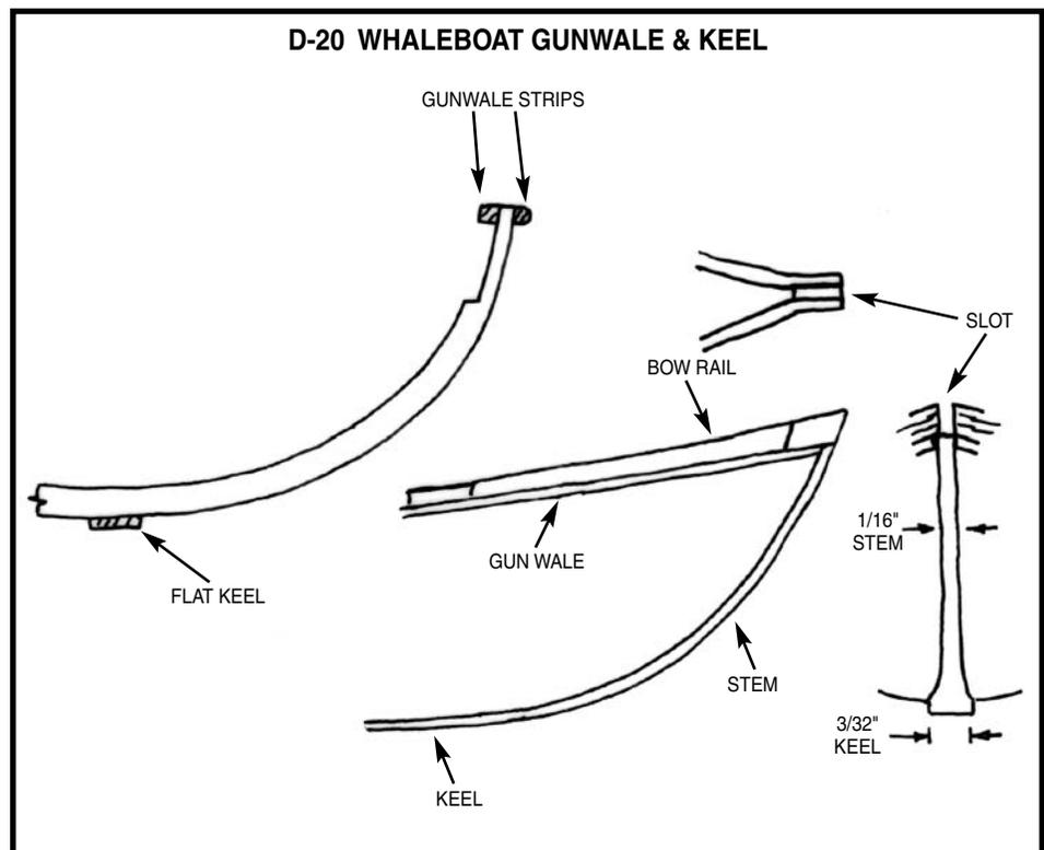
both and round the outboard strip. On top of the rail forward add the bow rails. The bow rail is open at the stem forming a slot. This is where a harpoon line would run after harpooning a whale (Figure D-20).
