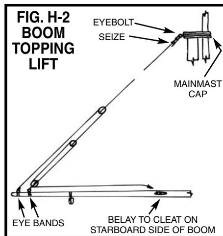
located forward of the sheet band. Rig the tackle, and for storage, run it along the boom and lash it to the boom. This tackle is an added support for the boom when under sail. When in use, the tackle would probably be hooked to a quarter bitt.
