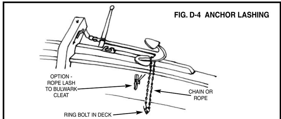
FIG. D-4 ANCHOR LASHING
