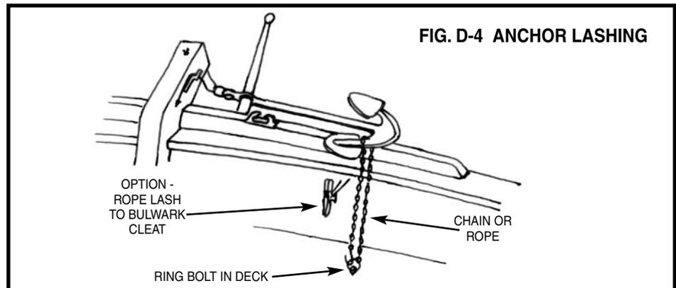
FIG. D-4 ANCHOR LASHING
