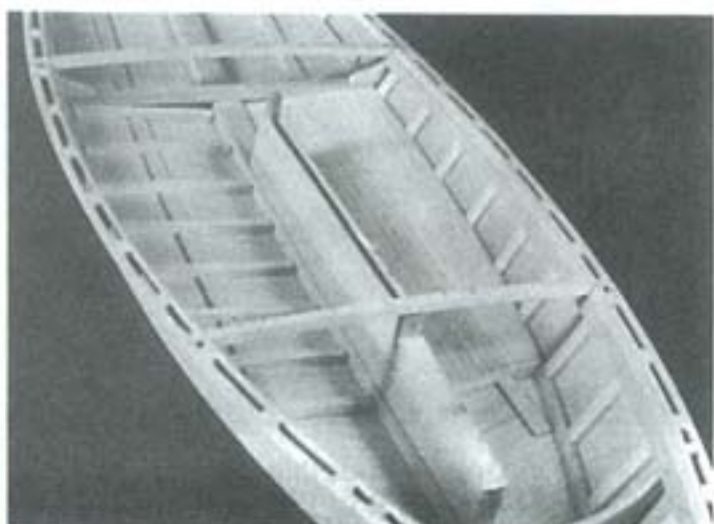
CEILING FLOORS FITTED AND CEILING PLANK LAID ON PORT SIDE.
