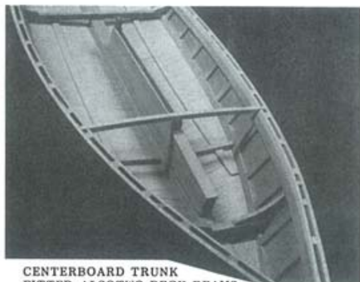
VIEW OF FORWARD STRONGBACK AND ITS KNEES. SPREADER HAS BEEN REMOVED.
