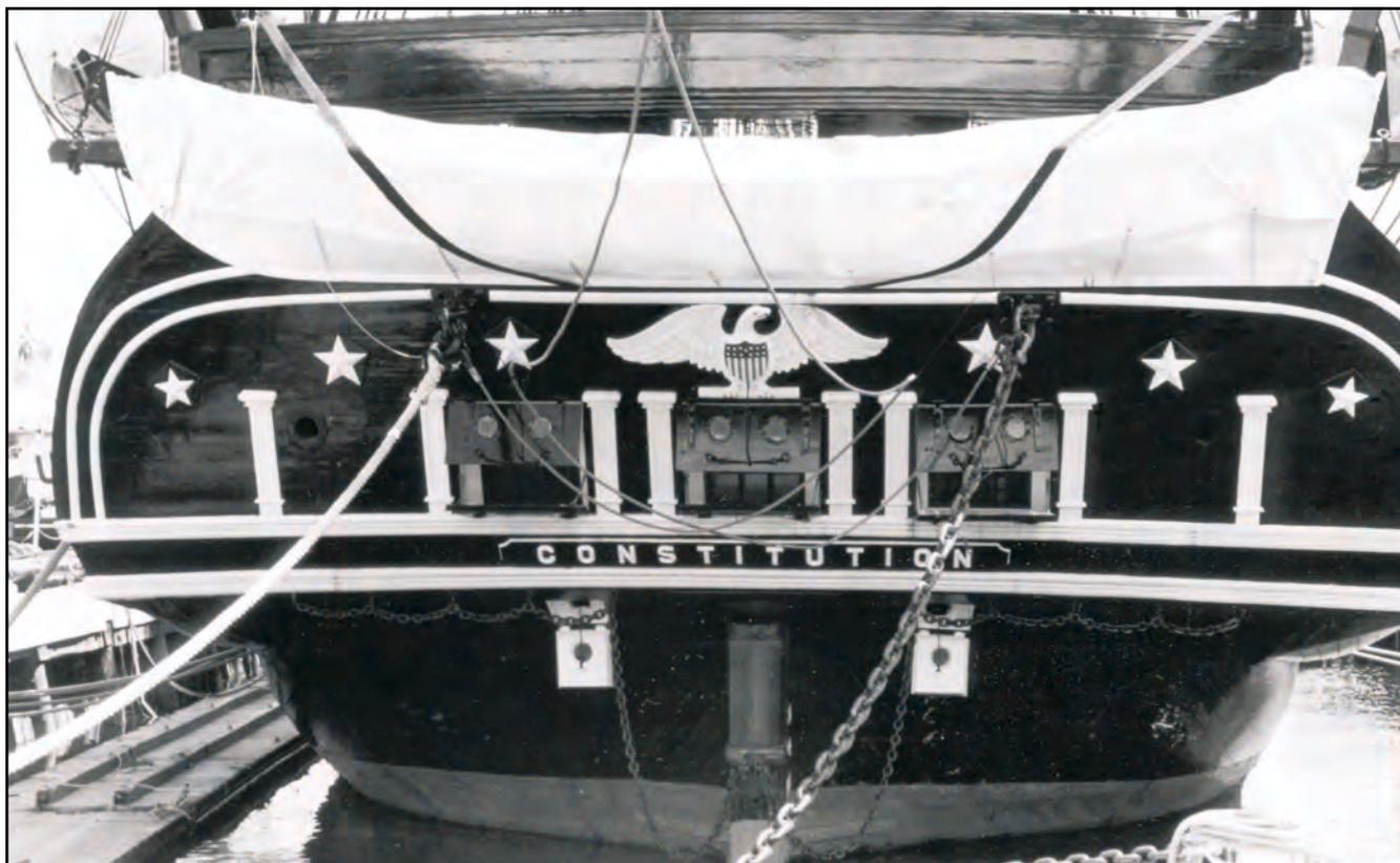
CAPTAIN'S 28-FOOT GIG is suspended above three chase ports with the bottom of their half lids lowered. Beneath the ship's name on either side of the rudder are the berth deck port lids.
