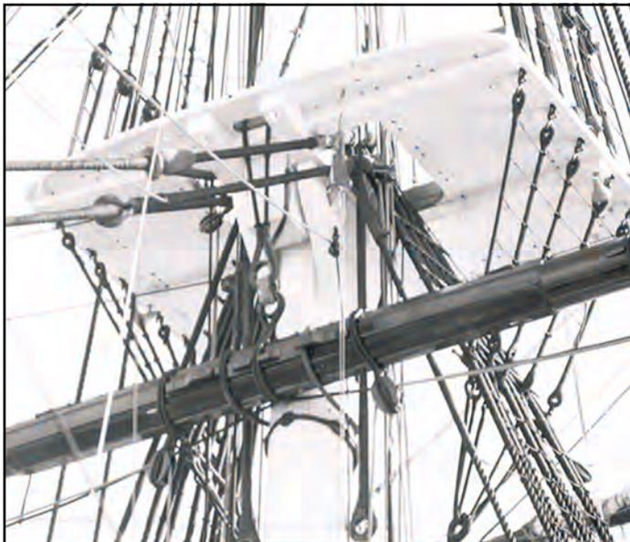
FORE YARD. Note sling detail and how the futtock shrouds lead down to the bentinck shroud ring.
