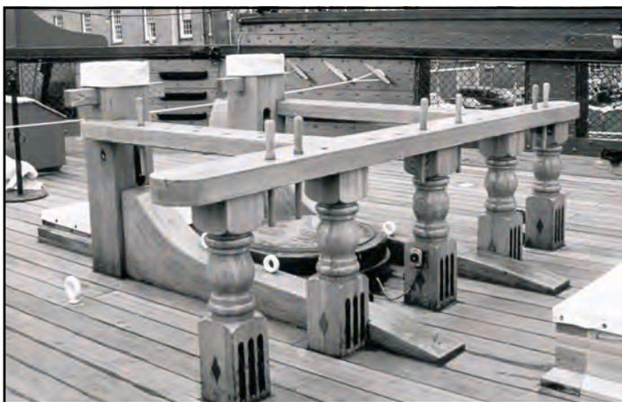
**FOREMAST FIFE RAIL** undergoes restoration. Note the triple sheaves in the base of each stanchion. Three levels in the bulwark are normally used for belaying large lines.
