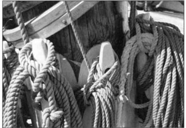
*Rigging lines belayed to fore mast cleats.*
