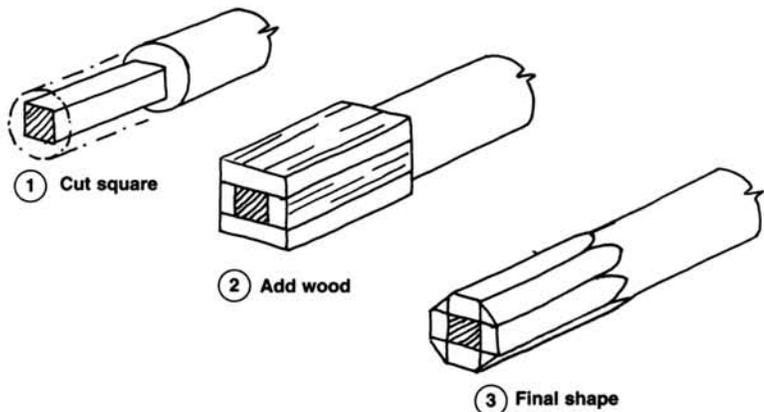
gon is equal to the diameter of the round part of the mast above. This means that the distance across the corners of the octagon is larger than the diameter of the round part of the mast. The dowel provided in the kit is 5/16" diameter, which is the diameter of the round part. If you cut the octagon into the dowel, the distance across the flats will be too small. On the other hand, since you will have a mass of cleats and belayed rigging lines in this area, you may not notice the difference.
