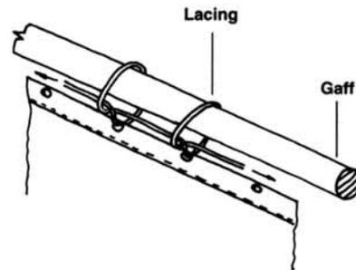
FIG. 81 – Mainsail In Hand—Ready To Install
