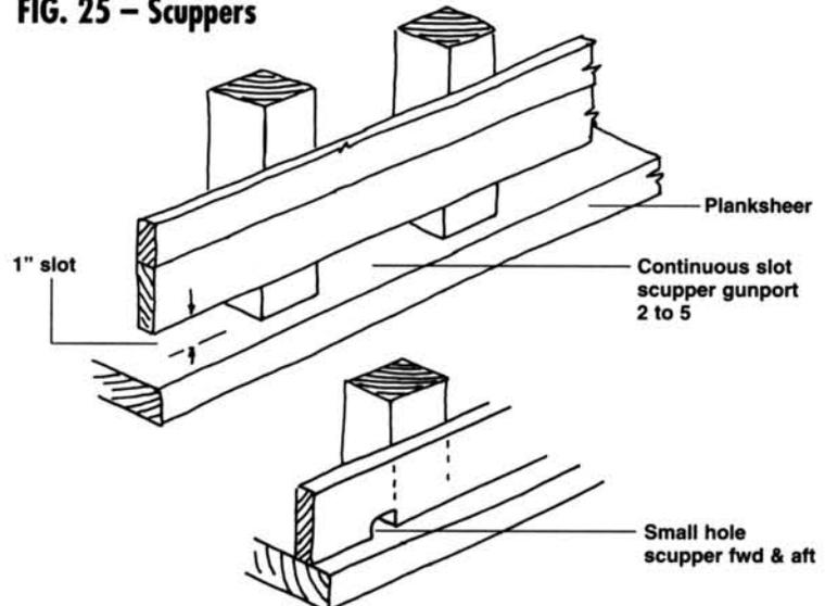
The top 3/64" plank should continue across the gunports. Apply a 1/32"-square vertical strip of wood on each side of the gunport, simply to cover the end grain of the bulwark plank (you could omit this on the model).
