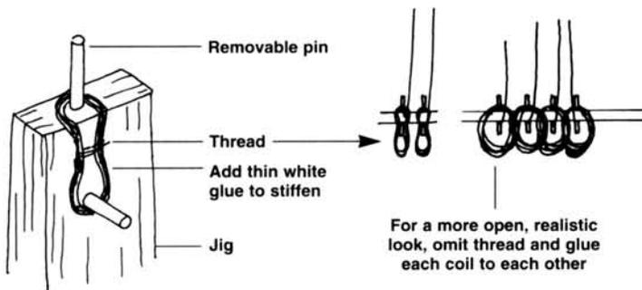
At 3/16" model scale, it's easier to add coils on pins separately from belayed line
