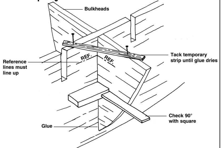
**FIG. 6 – Applying Battens**
