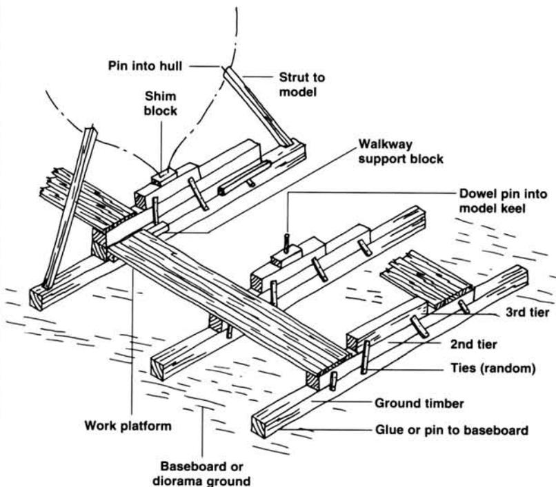
**Note:** Shim model so the load waterline is parallel with the baseboard. See plan sheet 3 for complete mounting plan and dimensions.
