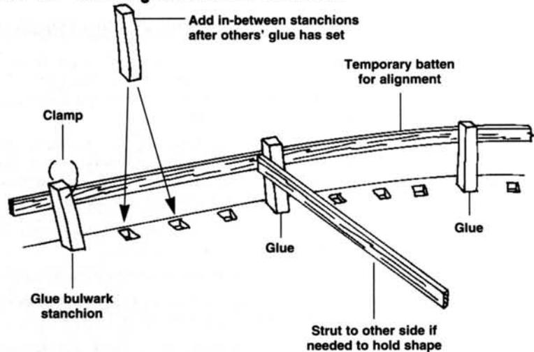
**FIG. 12 – Installing the Hawse Timbers**
