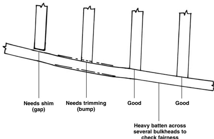
**FIG. 9 – Installing the Transom Framing**
