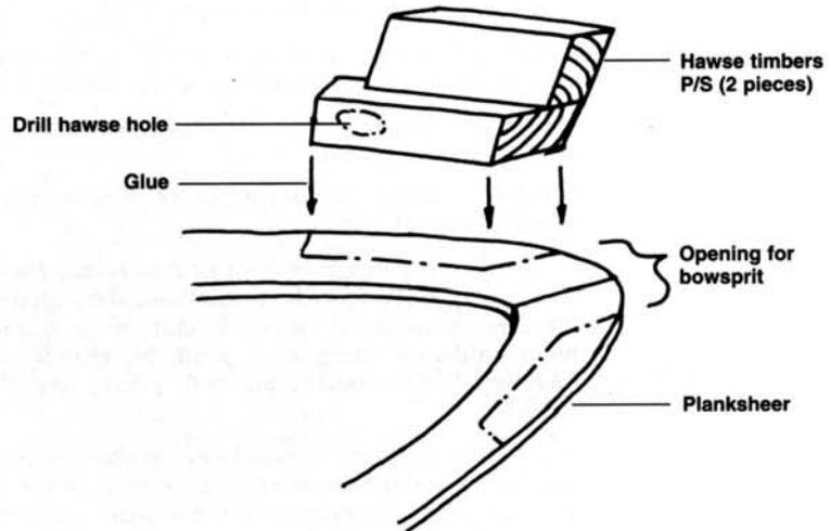
**FIG. 13 – Installing the Main Rail**
