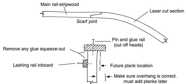
**Fig. 1-13 Installing the Topgallent & Log Rail**
