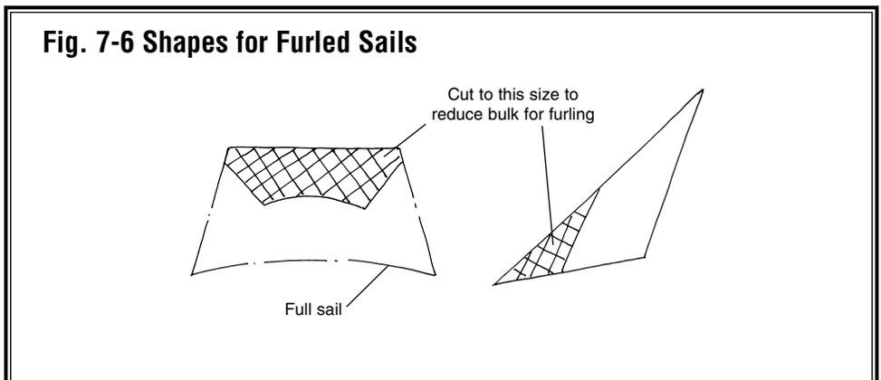
sails may require being reduced by one-third. Test first to see how much material is required for a neat, tight furl.
