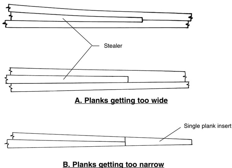
**Fig. 2-2 Staggering the Planking Butts**
