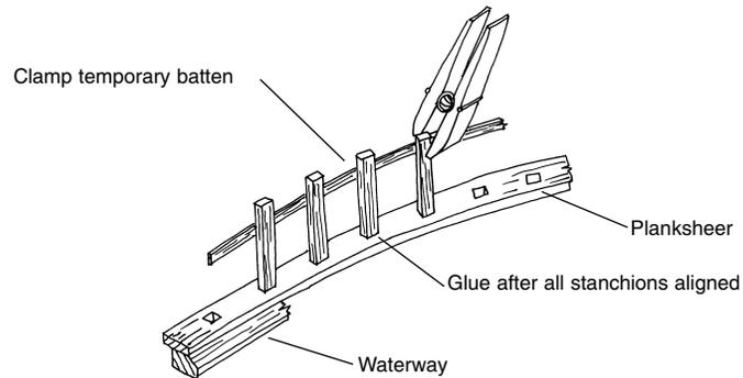
**Fig. 1-12 Installing the Main Rail & Lashing Rail**
