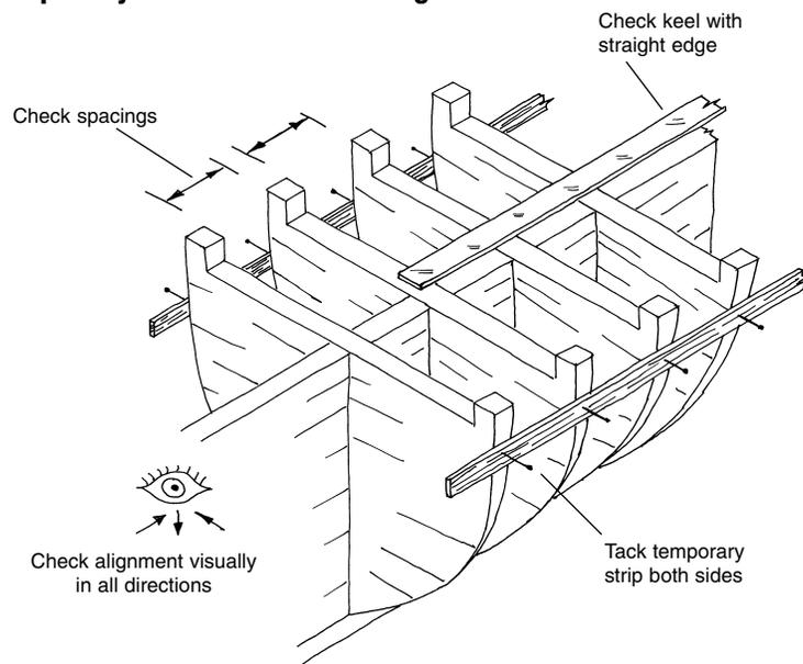
**Fig. 1-7 Correcting Bulkheads at Bearding Line**
