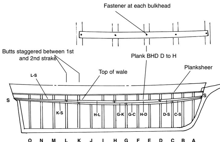
**Fig. 2-6 Installing the Fashion Piece at Stern**
