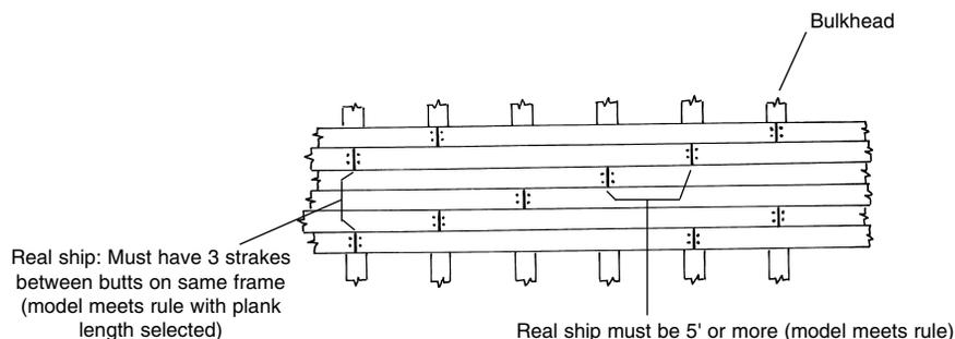
**Fig. 2-3 Spiling the Planks When Edge Bending Cannot be Accomplished**
