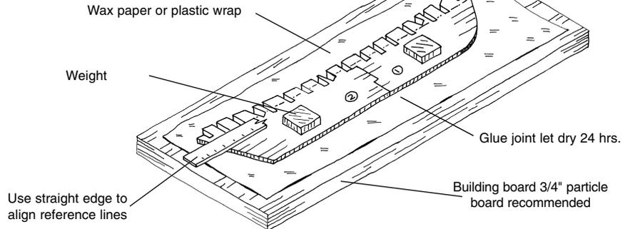
Fig. 1-2 Installing the Keel, Stem & Sternpost
