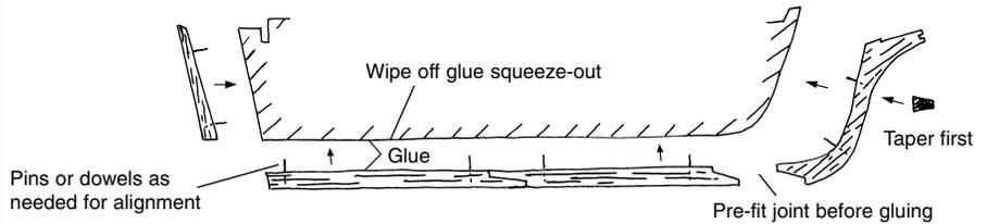
Fig. 1-3 Cutting the Rabbet into each side of Center Keel
