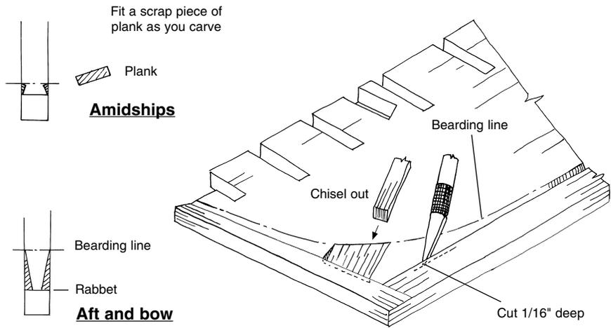
Fig. 1-4 Cutting Bulkhead Bevels
