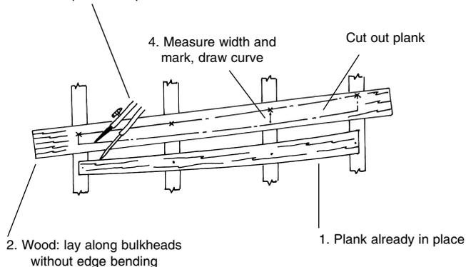
Planking will require tapering fore and aft from the top of the wale down to the keel. Consequently, the hull below the wale is divided into **Belts A** through **D**.
