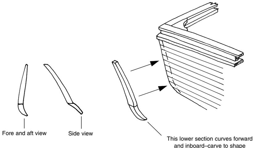
*Side Planking Above the Wale:* Planking is  $3/64$ " thick from the top of the wale to the planksheer. From planksheer to main rail, it is  $1/32$ " thick. These planks are fairly uniform in width from bow to stern and can be easily fitted.
