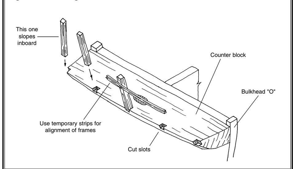
**Fig. 1-10 Installing the Bow Filler Block**
