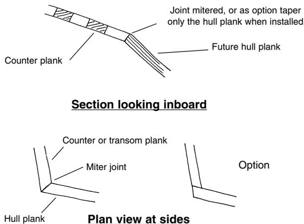
**Fig. 2-5 Installing First 2 Strakes in Belt A**
