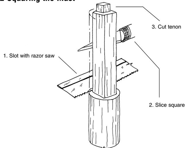
**Fig. 6-3 Fid in Topmast Heel**
