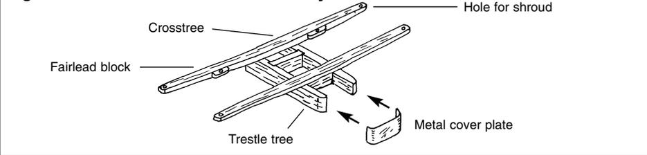
rigging. Assemble the cap and jibboom on the bowsprit. Be careful and align it correctly before gluing. Mortise the aft end of the jibboom into the block at the bow as shown on the plans.
