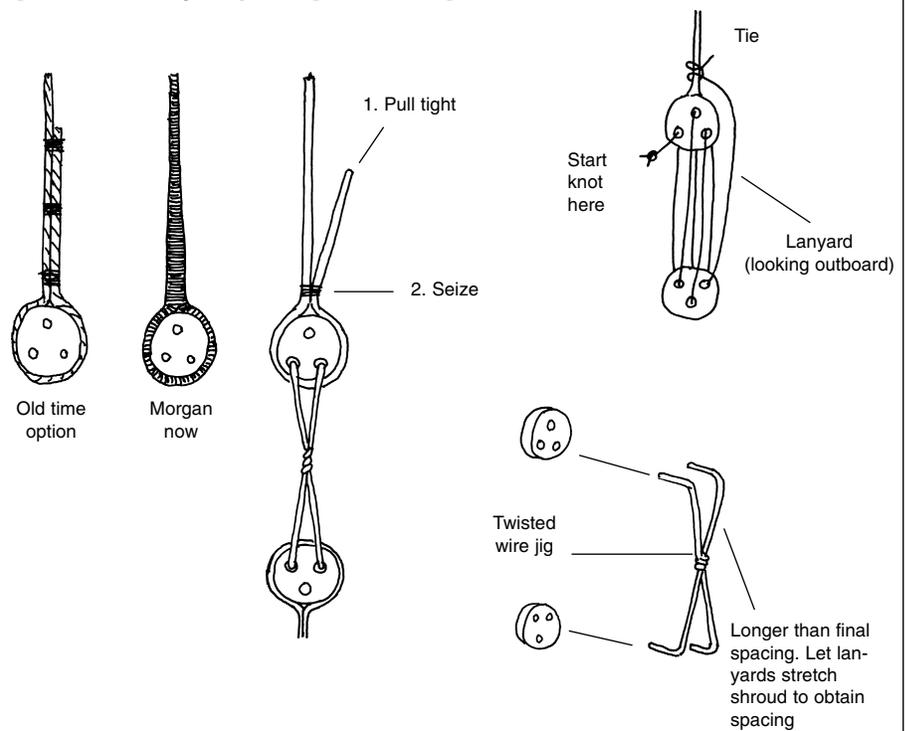
Instead of chainplates, the topmasts have deadeyes and futtock shrouds (Figure 8-3). Make the futtock shrouds from brass wire. *Note:* Topgallant shrouds have bullseyes, but the royal mast has no iron futtock shrouds, deadeyes, or bullseyes. Its shrouds pass through the crosstrees and set up with a lanyard at the futtock band.
