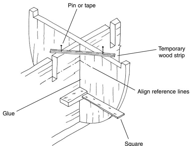
**Fig. 1-6 Temporary Battens for Hull Alignment**
