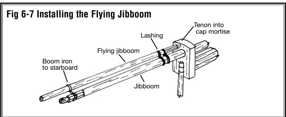
The jibboom begins as an octagon, becomes round, then returns to an octagon. Drill the required sheave holes. The jibboom passes through a hole in the cap and lashes to a saddle on the bowsprit. The flying jibboom is mostly round with a short octagon section at the end. Mount it starboard of the bowsprit so the stays can pass around the end of the jibboom. An iron at the end of the jibboom secures the flying jibboom, while a tenon in its heel fits a mortise in the bowsprit cap (Figure 6-7).
