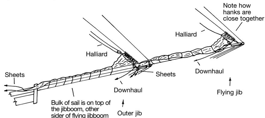
*No Sails:* Attach halliards to the downhauls and lead them to the end of the bowsprit (Figure 9-1). Halliard runs are identical to a rig with sails except for the head block's location. Remove sheets with the sails. If left on deck, they tend to clutter a model. Also, don't put hanks on the stays.
