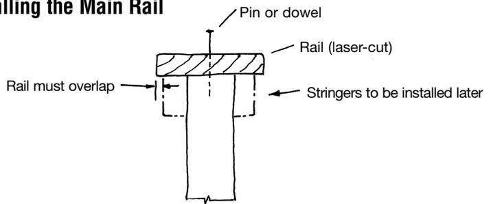
**Fig 1-13 Installing the Chock Rail**
