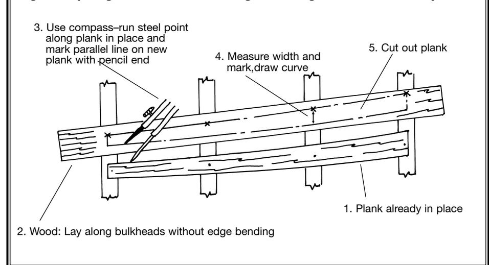
Another approach is to apply cyano to the edge of a plank already in place and on the bulkheads above it. Spray or brush the cyano's accelerator on the plank to be installed, then hold it in place. The glue sets instantly and no clamps are necessary. However, be sure to position the plank correctly the first time, because there isn't a second chance.
