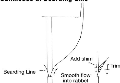
**Fig 1-8 Checking Hull Fairness with a Batten**
