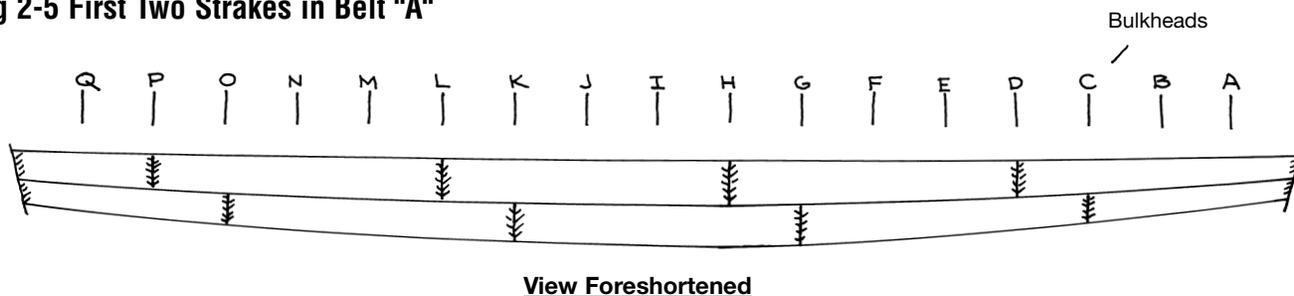
Install the planks. Repeat the process for the next strake, but stagger the butts. Install a plank from:
