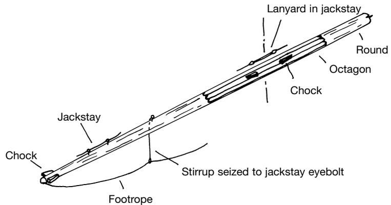
**Fig 6-10 Topsail and Topgallant Yard Parrel**
