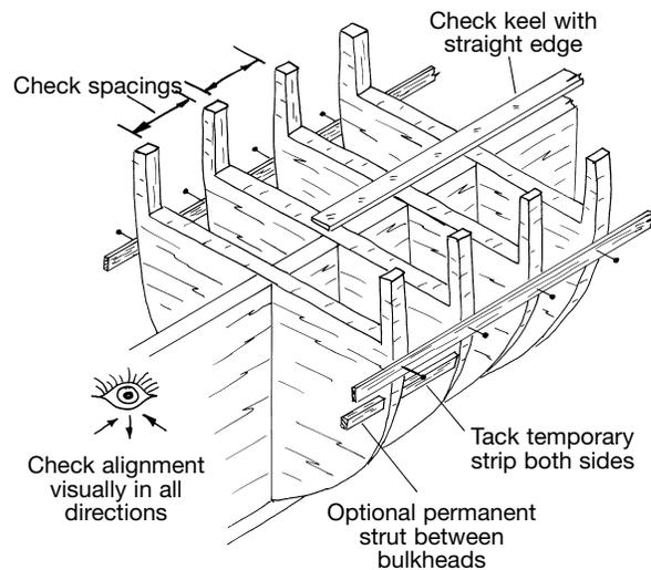
**Fig 1-7 Correcting Bulkheads at Bearding Line**
