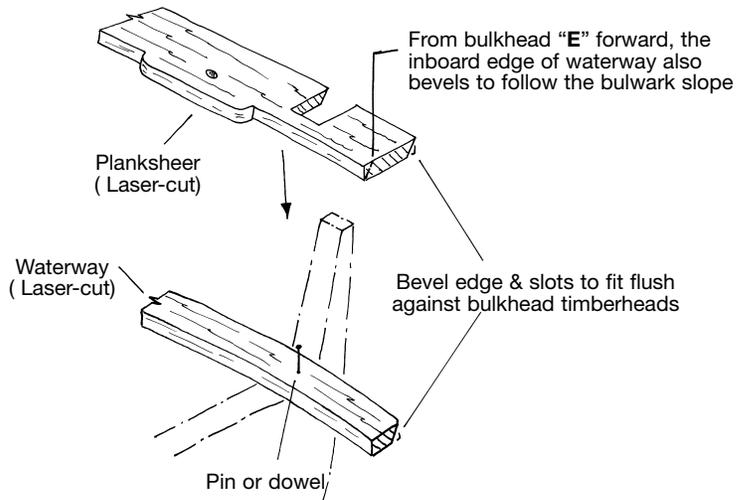
**Fig 1-11 Installing Knightheads and Timberheads at Bow**
