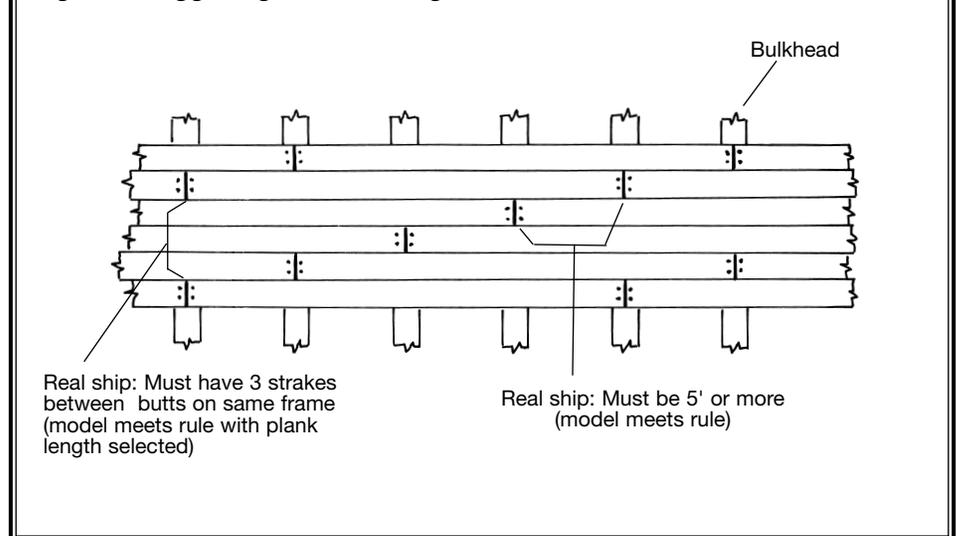
Fig 2-3 Spiling the Planks When Edge Bending Cannot be Accomplished
