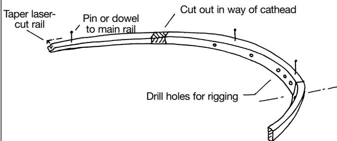
**Fig 1-14 Framing Around Gun and Sweep Ports**
