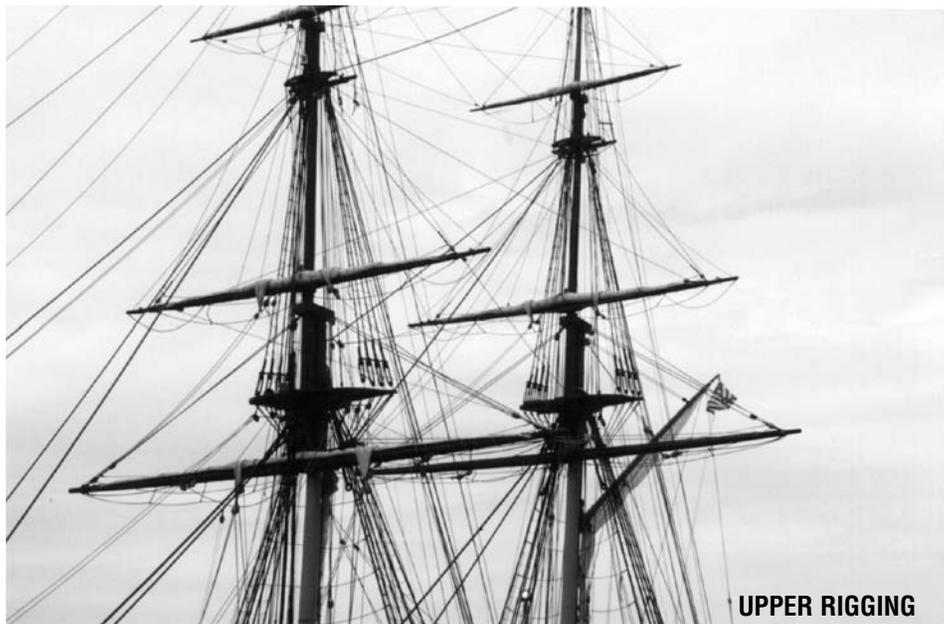
*Stays and Backstays:* Lines supporting the masts from fore and aft forces. A *running backstay* has a movable tackle on deck.
