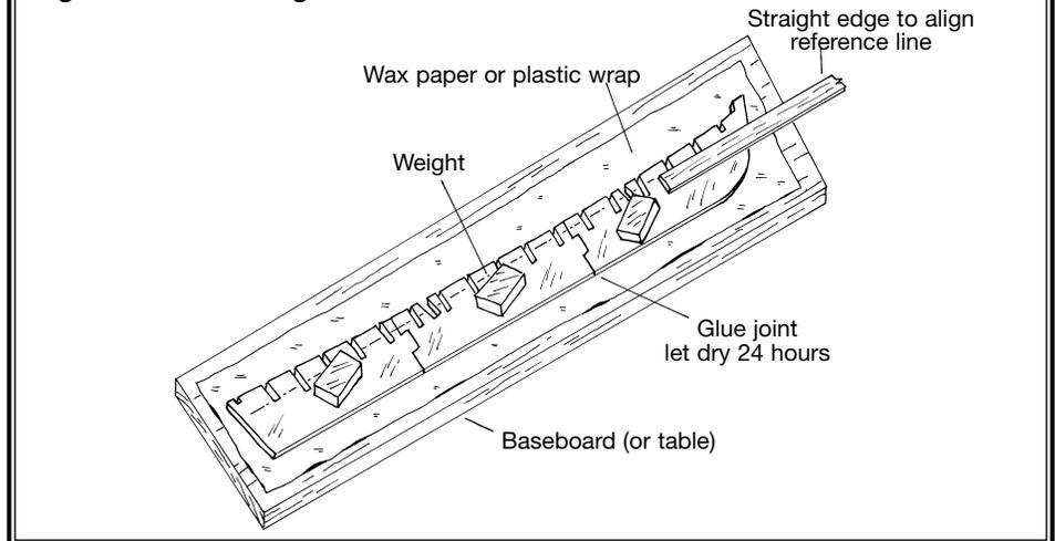
Fig 1-2 Installing Stem, Keel, and Sternpost
