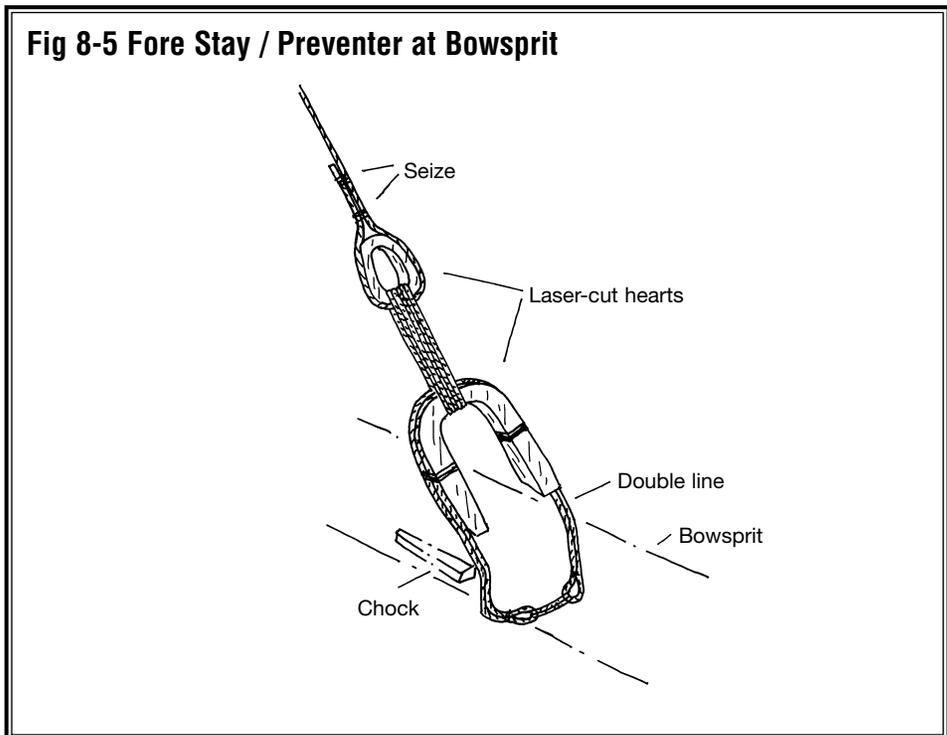
sets up to laser-cut hearts and an eyebolt on the starboard bowsprit bitt. The chock on the foremast bends the stay down, while applying tension.
