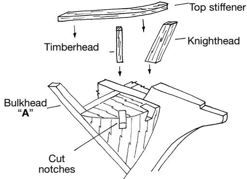
**Fig 1-12 Installing the Main Rail**
