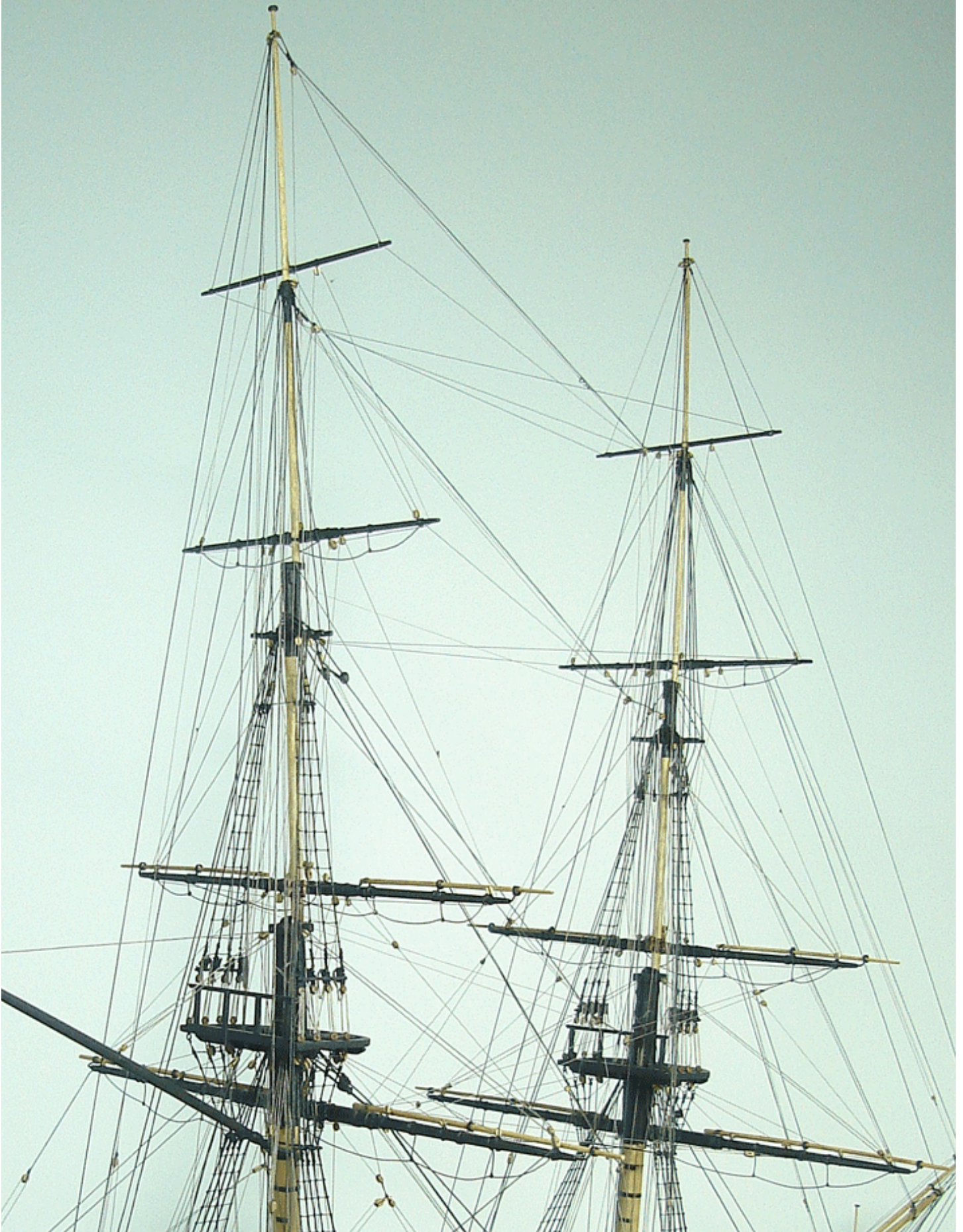
Topsail, Topgallant and royal yards rigging completed
