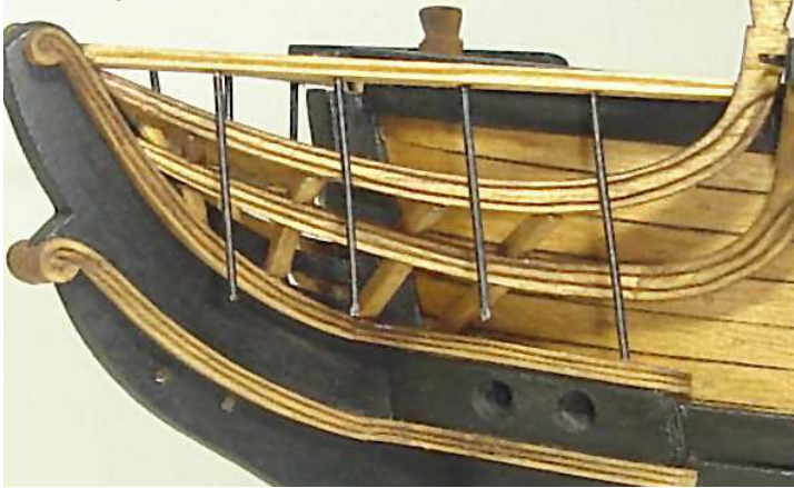
Step 5B - After cutting the stanchions to length the top rail is glued into pre drilled holes along the upper rail.
