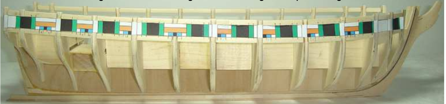
Marking the locations for the green frames using the template as a guide.
