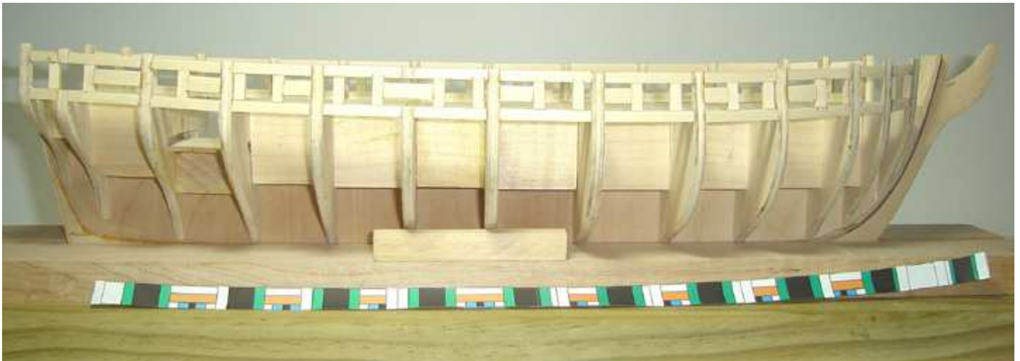
All of the red frames are glued into place. These frames define the top of each sweep port.
