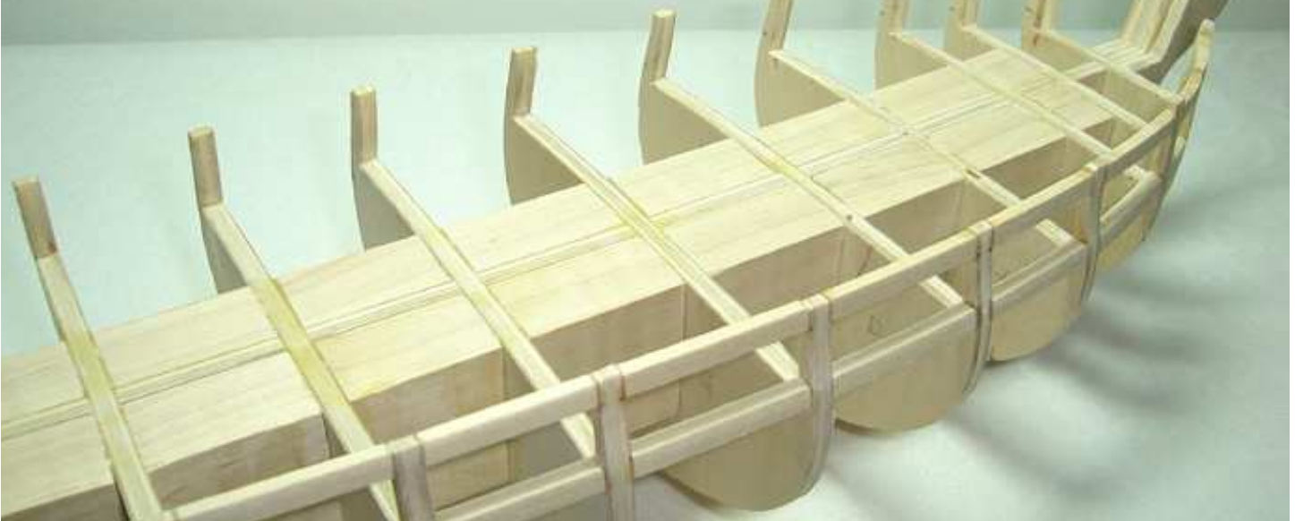
Gun port sill and lintel faired at the bow. Notice the graceful curve established.
