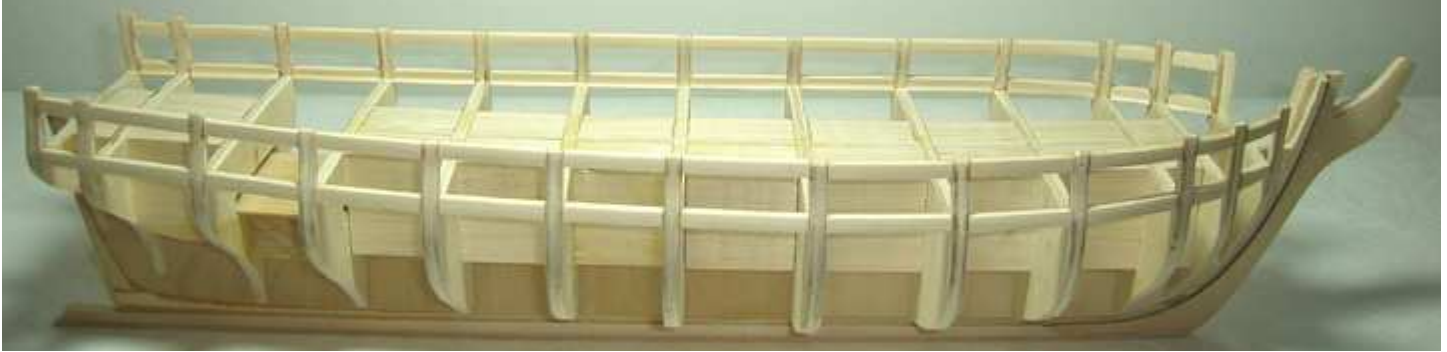
Gun port sills and lintels are completed.
