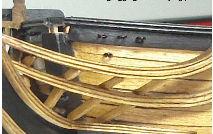
Step 5A - Place four eye bolts on the bow as shown on the standing rigging and belaying plans.
