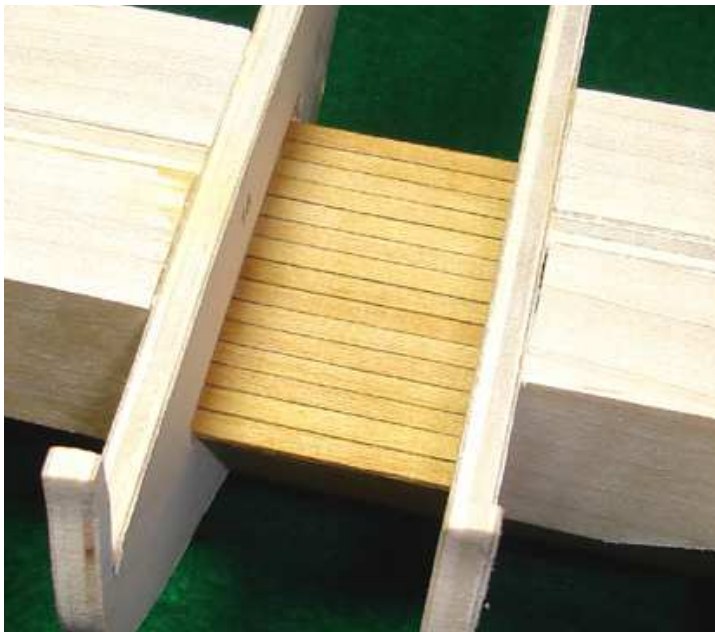
The planking between bulkheads 16 and 20 is completed. It creates a platform to simulate the lower deck which will be visible through the open companionway.
