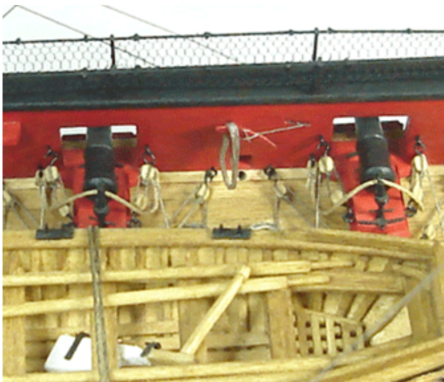
These two photos show the inboard portions of the main course sheets and braces (below) and the fore sheet (above). It is best if you add these soon before getting to much rigging done. It will be easier to complete them with less rigging to get in the way. Not shown is the main tack which is handled in the same way.
