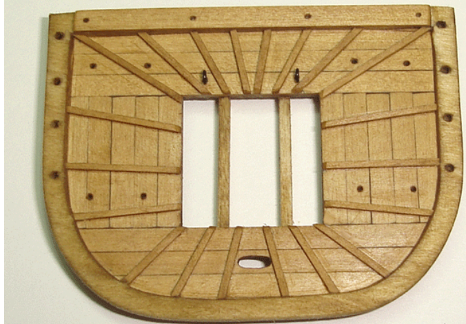
Fore top w/holes drilled. Note two eye bolts for stays.
