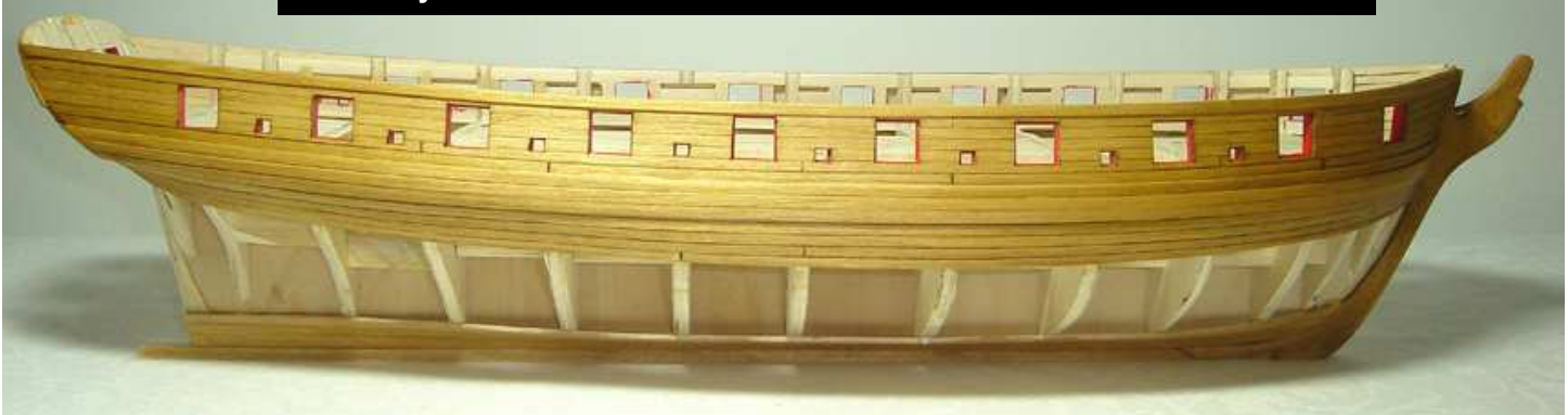
Second layer of the wales and the sheer strake have been added to the model.
