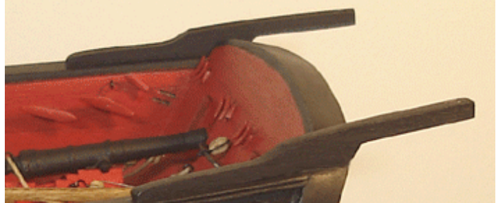
Stern davits in place, The cleats have not been glued into position yet.
