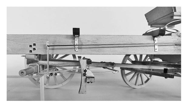
Slip on the remaining wheel and secure the wheels by gluing the pin of the cast wheel hub nuts and washers into the holes at the axle ends. The wheels can be left to turn freely or be glued to the axle to keep your display model from rolling on the shelf.
