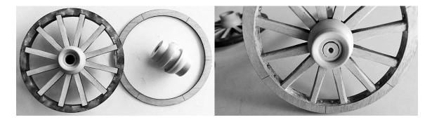
Insert the arced end of the spokes in the hubs. The correct number will fit snugly into the center of each hub. Drop the spoke subassembly into the notches within the appropriate wheel rim. Twist the hub slightly to correct any misalignment of the spokes. Opposing spokes should form a straight line. Laminate the other face in place to lock in the spokes. Be sure that the fellows scoring lines up with the already laminated faces.
