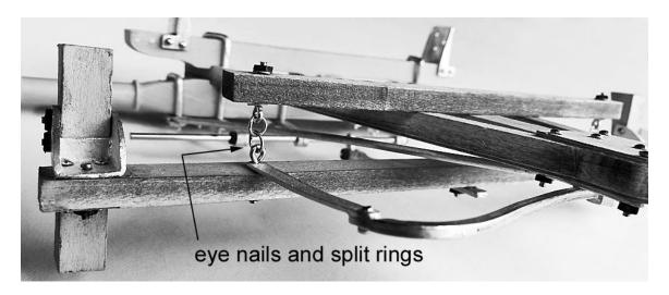
Slip the rear wheels on their axle and use them to position the brake shoe brackets on the brake arm. The midline of the brake shoes is approximately 7/32" from either end of the
