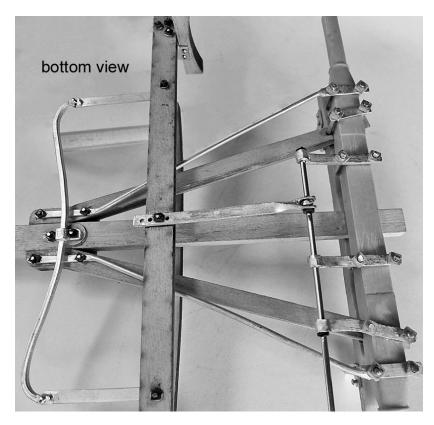
NOTE: the center bracket on the return spring faces up so it will lie flat against the round spring spacer. The eyes in the eyebolts face the tabs on the return spring arm.
