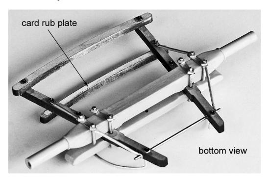
Measure out 7/8" forward at a right angle to the front face of the axle and mark each brace. Drill a 1/16" hole through each wood brace so a brass rod slipped through the holes will be parallel to the axle. The distance from the inside (square) end of either brace to the outside of the brass rod should be 7/16".
