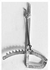
Place the Geisler brake lever casting ratchet side down. Note the holes in the release handle near the top and in the ratchet pawl at the arced section. Make a small right-angle bend in the end of the 1/32" brass rod. Insert the bent end in either hole, Measure to the other hole and make an identical bend in the brass rod. This will connect the release lever to the pawl. Trim the bent ends so they barely protrude from the other side. Glue in place
