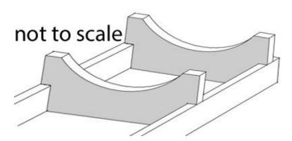
Assemble the construction cradle by gluing two rails made from 3/16" x 5/8" x 12" kit lumber to the rectangular cutouts in the two laser cut cradles. Position one cradle in about 1/2" from one end of the rails. This is the rear. Position the other cradle 7" farther along from the rear
