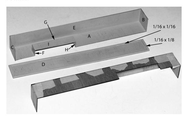
Glue a length of 1/16" x 1/16" kit lumber to the face of door **D** along the top and bottom edges. When dry round over the outside edge of the added strips and fill in between them with short lengths of 1/16" x 1/8" kit lumber (1/8" sides against part **D**).
