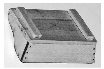
Assemble the seat sides and back, maintaining right angles between them. Because they are angled from the vertical, the bottom edges will not be flat. After reinforcing this with brass nails, per the photograph, carefully sand the bottom flat.
