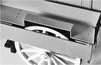
The pannier is secured by three small brass nails into each cradle arm that are spaced outward from the inner back wall at approximately 1/8", 3/8" and 5/8". #74 pilot holes must be drilled through the pannier and into each cradle arm. It is recommended that you then use a #66 drill to make clearance holes in the pannier only. BE VERY CAREFUL NOT TO DRILL THROUGH THE CRADLE ARMS. The outer two of each group of
