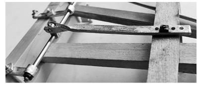
Use an escutcheon pin to attach the brake coupler to the actuator, left hanging on the brass rod. Secure the pin with a gasket square nut so that the joints, for now, swing freely. Insert an escutcheon pin through a card washer and then through the center hole in the top side of the of the brake arm and use it to secure the brake coupler to the brake arm through the second hole in the coupler, per the photograph. Coupler and arm may be glued together at a 90° angle.
