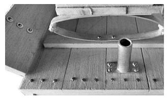
before. Re-install the lever guide in the same manner, including use of smallhole gasket washers.
