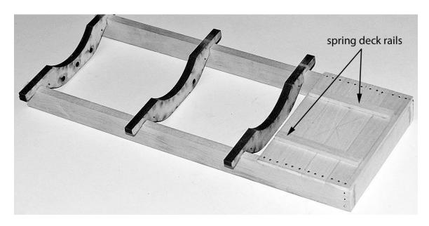
Measure 2 3/8" forward from the rear end of the rails and draw a mark. Unpin one of the bed brackets from the undercarriage, center it on the pencil line, per the following photograph, mark and drill holes for escutcheon pins. Do this on both sides. Re-pin the bed bracket to the undercarriage.
