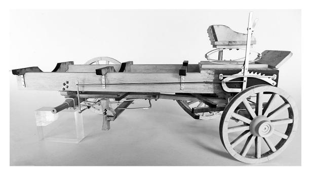
Pull the bed rail pins tight and finish off with a card washer and gasket nut for each escutcheon pin. Pull tight the loose pins holding the bed brackets to the chair and finish off with gasket nuts. Trim off the excess length from all of the escutcheon pins. Slip on the wheels, excepting the right rear. Use whatever fits to support the right rear axle.
