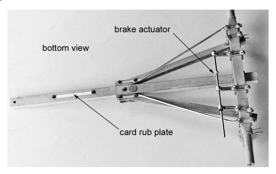
Secure the left-hand large U-bolt with a U-bolt plate and two cast nuts. Slip the angle shaft mount over the right-hand large U-bolt, but do not yet secure it. Slip a small U-bolt around the axle only on either side of the coupler and tape the three loose U-bolts in place. Refer to the middle photograph in this section for guidance. Slip a straight shaft
