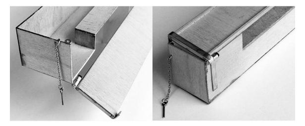
Referring to the above photographs, glue the door hinge halves flush with the edges of the door, on the outside. Escutcheon pin the bottom hinge halves to the door hinge halves to align them and glue in place under A. NOTE: the cylinder part of the bottom hinge hangs down. Glue a gasket nut onto the escutcheon pins against the hinge cylinders, then cut the pins so they protrude slightly from the nuts.
