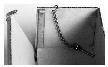
Glue a pin bracket to each end so it aligns with the bottom, NOT the outside edge of the sides. When the door is closed the tab on its hinge should lap over the bracket with the holes aligned.
