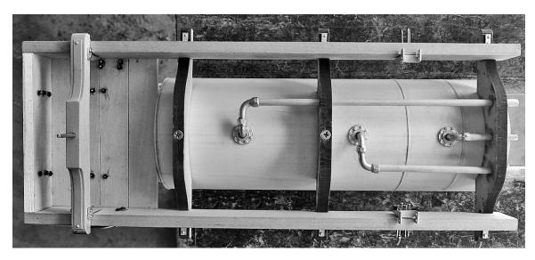
Insert the 5/32" pipe dowels. Measure out 3/8" on each dowel from the outside of the rear tank cradle. (They will measure approximately 5 3/4", 1 3/16" and 3 3/16".) Remove the pipes, paint them orange and glue them in place.
