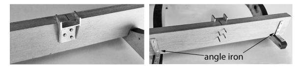
Maneuver the coupler between the front running gear arcs and into the space between the front axle and half chair. Pin the two sections together by inserting the kingpin and pivot chair. Slip on all four wheels. Temporarily pin the bed rails to the rear undercarriage brackets. Where the rails lie against the forward bed brackets, mark the four pin holes on each rail. Unpin the bed and drill the holes.
