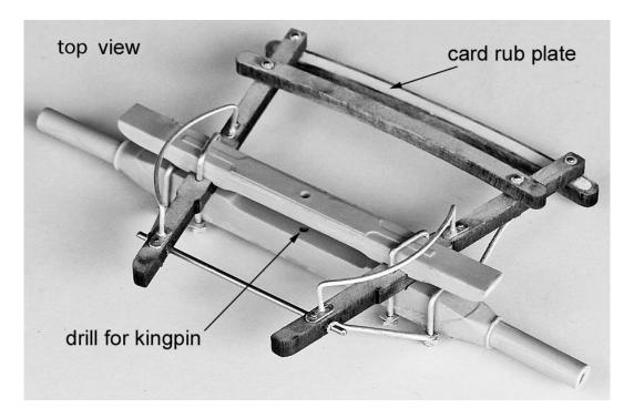
Use the kingpin hole in the half chair to mark the front axle for drilling. Remove the tape and drill a 3/32" hole ALMOST through the axle. Put it all back together and secure the U-bolts with U-bolt plates and cast nuts.
